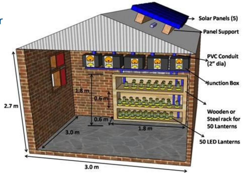
A typical Solar Charging Station
