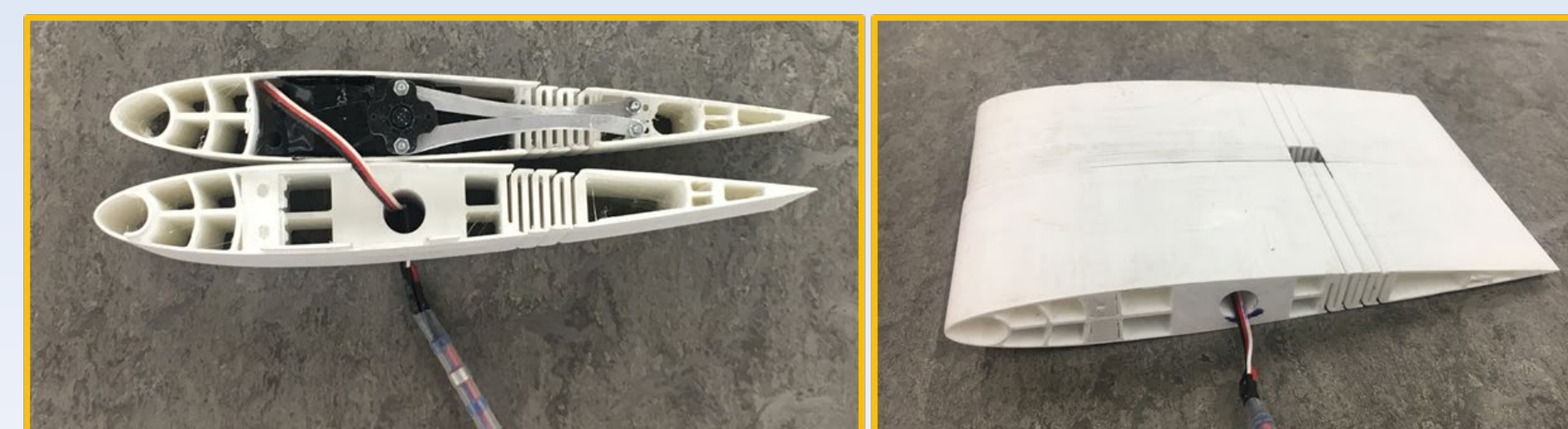
Figure 2. Engineer the nature for sustainable development: a 3D printed morphing wing prototype. The morphing wing concept presents great potential to improve aerodynamic efficiency of future fuel-efficient civil aircraft.
