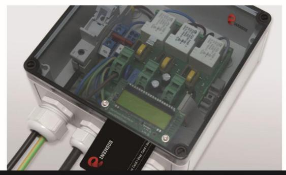
MPM for rural electrification: Prepaid meter and limiter of both energy and power with integrated load management used in micro-grids.
